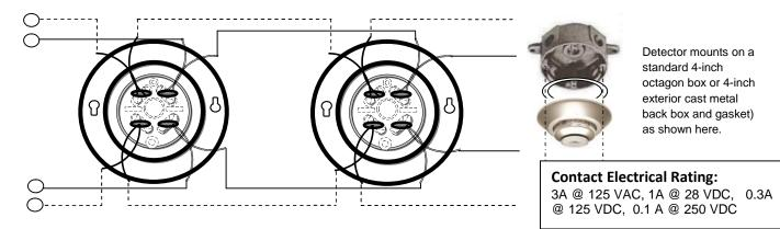
**CAUTION**: All wiring must be installed in compliance with the local electrical code using approved cable, AWG 18 minimum. Begin electrical connections by stripping approximately 1 in (2.5 cm) from the end of each wire. Insert the stripped end into the wire retaining hole in the terminal bar, wrap clockwise around the terminal screw, and tighten. Circuit wiring must be broken at each terminal to ensure proper supervision.
