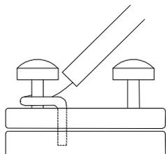
All wiring must be installed in compliance with the local Electrical Code using approved cable, AWG 22 minimum. Begin electrical connections by stripping approximately 1" (2.5 cm.) from the end of each wire. Insert the stripped end into the wire-retaining hole in the terminal bar, wrap clockwise around the terminal screw, and tighten.
